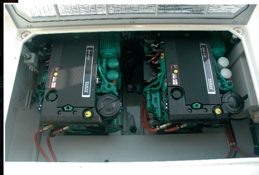
(Above) The test boat contained two Volvo D4 diesels. (Left) The dash is well laid out with nicely-positioned gauges and engine controls.
